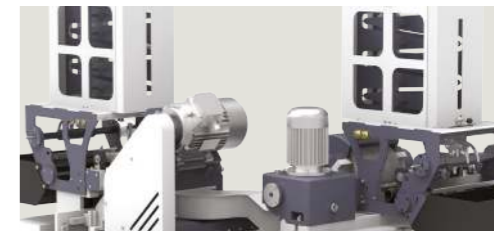
Grinding of R/F & S/F with Auto feeding - 2 Unit
